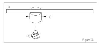
**2.2** Place the fixing plate on the fixing point, lining the screw holes up with the horizontal and vertical lines.
